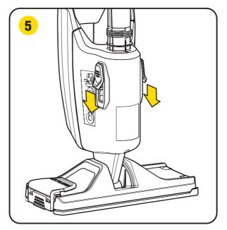
Then, while still under running water, pump the yellow Cleaning Levers to flush water through the mechanism. Continue until the rinsed water is completely clear.
