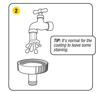
Rinse the Dispensing Nozzle until the valve is clean and the water runs completely clear.
