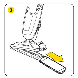
Remove the EasyDeck Applicator Pad and leave to soak, then rinse under running water until the water runs clear and the pad returns to it's original colour.
