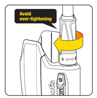
Insert the Pole into the Applicator Body and twist the Collar clockwise until the Pole is securely attached.
