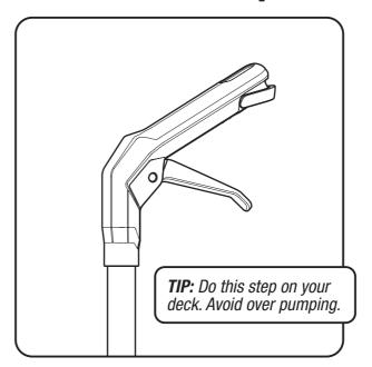
Unhook the Trigger and squeeze the handle 6-10 times to begin product flow.
