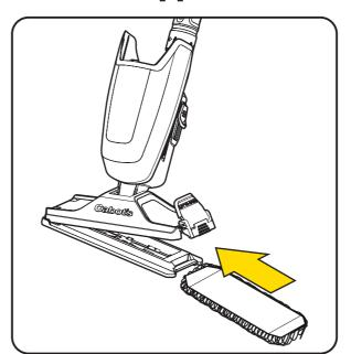
Open the Latch on the Applicator Body and slide a clean EasyDeck Applicator Pad onto the Applicator Base.
