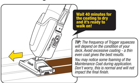
For best results, use long, smooth strokes along the direction of the boards. Squeeze the Trigger as needed to achieve a consistent and light coating.
