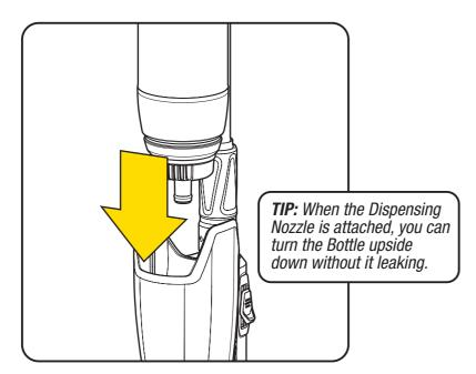
Place the EasyDeck Bottle into the Applicator Body and press down firmly.
