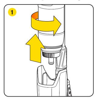
Twist and remove the EasyDeck Bottle from the Applicator Body vertically without tilting to avoid ejection of the silicon seal from the Dispensing Nozzle and prevent spillage. Replace the Dispensing Nozzle with the Bottle Cap. Unused EasyDeck coating can be stored upright in a cool, dry area for up to a year.
