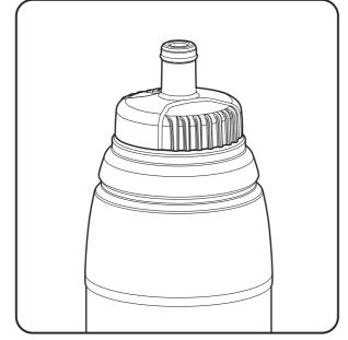
Replace Bottle Cap with Dispensing Nozzle and ensure this is firmly screwed on.
