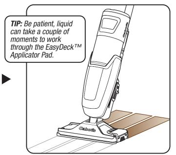
Ensure the EasyDeck Applicator Pad is saturated enough by moving the *Cabot's* EasyDeck over a small area of decking. Stop squeezing once it leaves a light even coating. If the area is over saturated, refrain from further pumps and begin coating.
