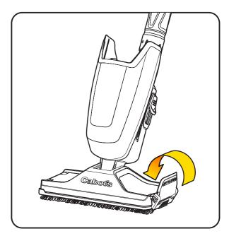
Close the Latch firmly ensuring the Applicator Base is clipped in.
